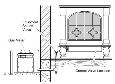
Figure 20 - Checking Gas Joints
